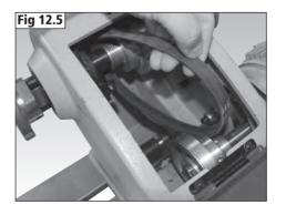
To remove the belt from the spindle pulley the spindle must be detached from the headstock.
