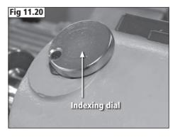
Disengage the spindle lock by lifting the indexing dial and rotating to a position where it is not located in the recess then lowering, **Fig 11.21**.
