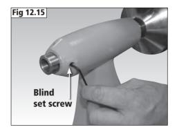
Remove the blind set screw from the hand wheel using a 3 mm hex wrench as shown in **Fig 12.16**.
