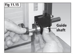
The rear guide must now be set in the correct position. Loosen the rear guide lock shown in **Fig 11.14** and position the guide by moving the guide shaft as shown in **Fig 11.16**.
