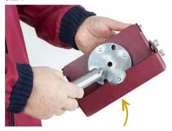
Turn the HollowPro™over to access the stem fitting location
