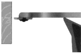
2. Always use the tool with the straight part of the shaft on the tool rest.
