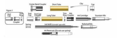
• Slide the clip onto the cap, then press them into the top of the upper barrel (shorter tube).
