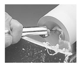
The Robert Sorby Thread Cutting tools are available in three thread sizes. These are 10, 16 and 20 threads per inch (TPI). The thread sizing gauge is a must have for anybody wanting to make accurate threaded boxes. There is also available a tool rest and a relief tool to assist in the internal thread cutting.
