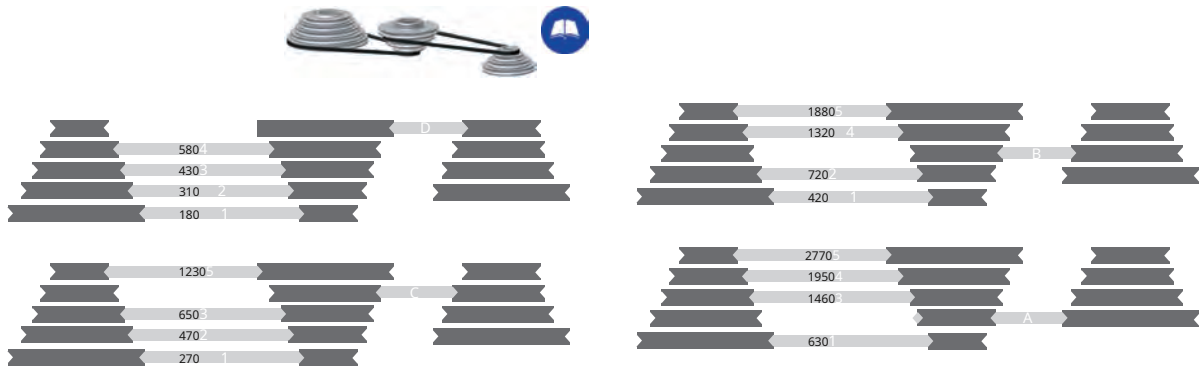
Fig.4-1: 50Hz sticker in the protective cover of the V-belts
