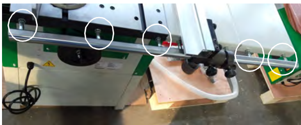
Fig. 8: Mount the stop guide rail
