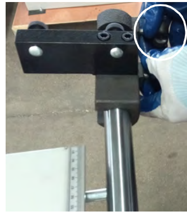
Fig. 9: Sliding the carrier onto the guide rail
