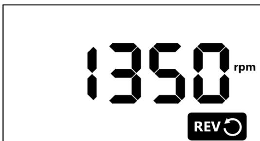
Speed Screen with Reverse Mode Engaged
