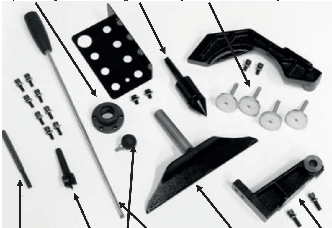
Removal tool Drive center Knock out rod Head stock bracket Tail stock knob Tool rest comes fitted to banjo
